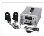
During the oil crisis of the 1970s, Hioki developed Japan's first clamp-on power meter to promote energy conservation. This innovation made power measurement safe and easy for all, leading to reduced electricity costs in factories and gaining overwhelming support from the industrial sector.
